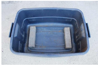
Figure 2. Two spacers set inside the bottom tote prevent the totes from sticking together.
