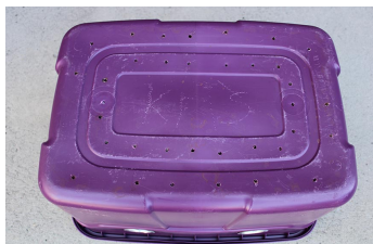
Figure 3. Twenty ¼-inch drainage holes drilled in the lowest form mold on the upper tote.
