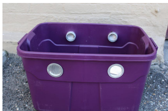
Figure 4. Fitted screen vents in predrilled holes.
